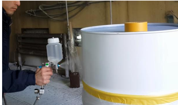
Applied Super Glass Barrier to Half the Surface (November 2013)
