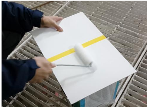
Applied Super Glass Barrier to Half the Surface (November 2013)
